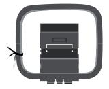
Release the tie-wrap and unwind the twisted lead. Fold the plastic stand forward through the loop frame.
