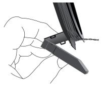
Push the tab into the open slot in the base of the stand. Press until the tab clicks home.
